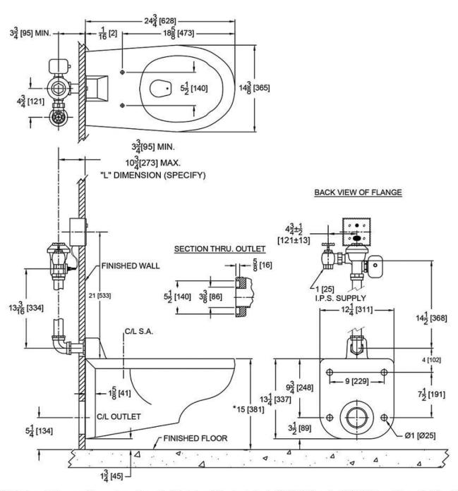
\*NOTE: For ADA compliance, top of seat height should be installed at 17" [431mm] - 19" [482mm] from finished floor.
