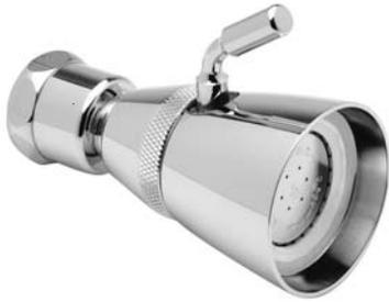
**ENGINEERING SPECIFICATIONS:** Self-cleaning brass shower head with hard chrome plated finish, brass chrome plated ball joint connector, maximum flow rate 1.25 GPM at 80 PSI, 1/2" NPT female threaded inlet, body width spray pattern adjusts from needle shower to heavy wash.
