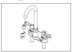
2B. (For faucets with optional cover plate). Align gasket with faucet bottom and press firmly together. Pass shank through cover plate and fasten to the faucet with the provided screws.
